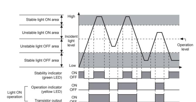
☒ The waveforms of 'Operation indicator' and 'Transistor output' are for Light ON operation. The waveforms are reversed for Dark ON operation.
