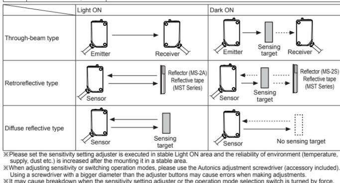
☒ Please set the sensitivity setting adjuster is executed in stable Light ON area and the reliability of environment (temperature, supply, dust etc.) is increased after the mounting it in a stable area.
