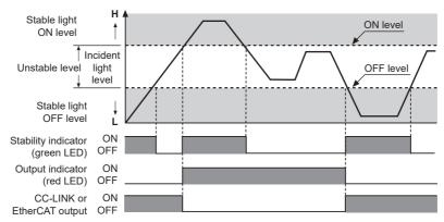
\*\*The waveforms of 'Operation indicator' and 'CC-LINK or EtherCAT output' are for Light ON. The waveforms are reversed for Dark ON.
