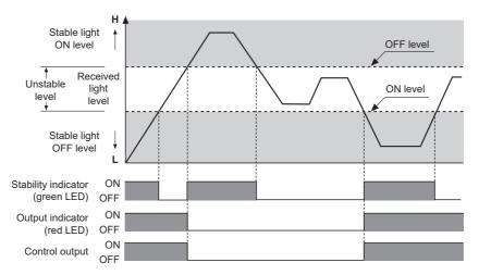
% The waveforms of 'Operation indicator' and 'Control output' are for Dark ON. The waveforms are reversed for Light ON.
