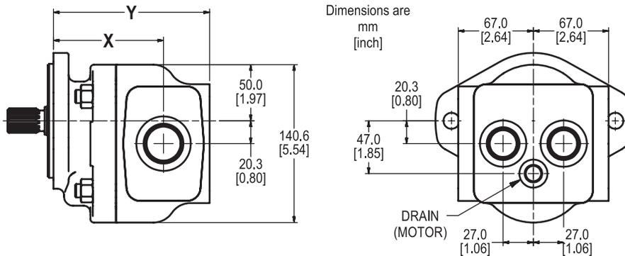
**PGP/PGM 620 Specification - Standard Displacements - Tandem Unit**
