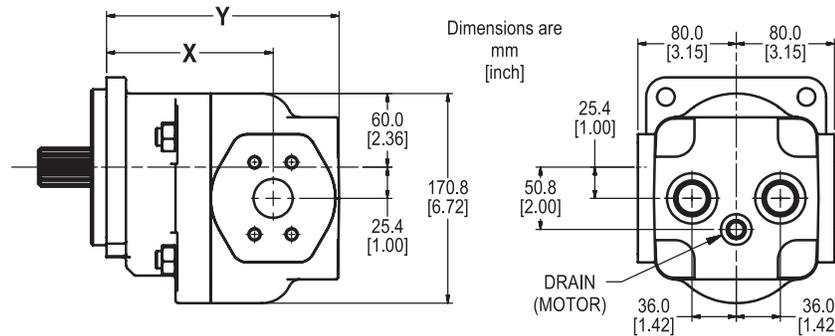
**PGP/PGM 640 Specification - Standard Displacements - Tandem Unit**
