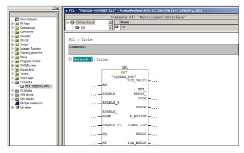
The function (here: PQDXXA-PROFINET-Z10 [FC1]) should be called in an organization block of type "Cyclic Interrupt" with a cycle time ≥ 10ms. Here an OB34 is used. The cycle time is set in the property dialog of the PLC in the HW Config program.
