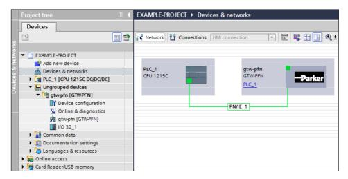
Check if the 32 byte I/O has been installed correctly under device and network (Device view).
