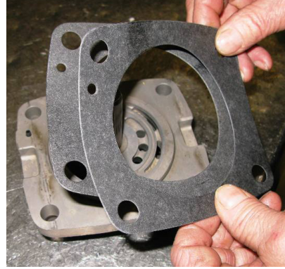
The number and thickness of gaskets determines the backlash
